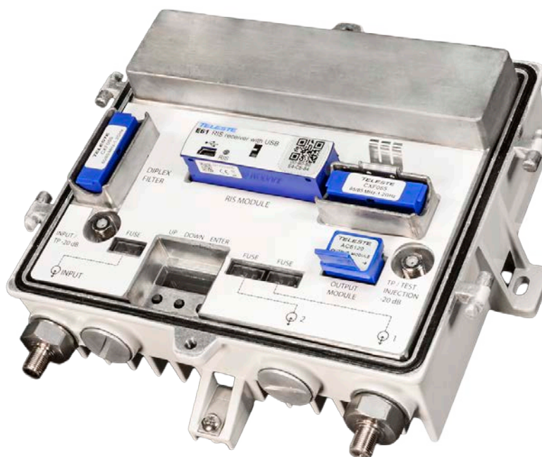
Figure 6. E61 installed into E3
